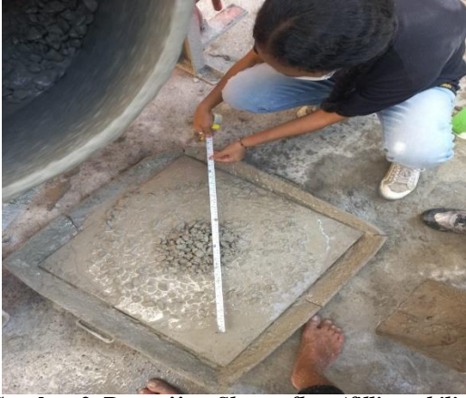
Gambar 2. Pengujian Slump-flow ( filling ability )
