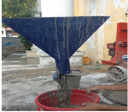
Gambar 5. Pengujian V-funnel at T5minutes ( passing ability )
