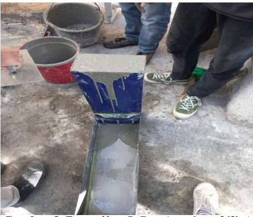
Gambar 3. Pengujian L-Box ( passing ability )
