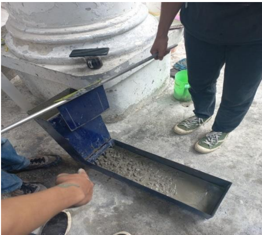
Gambar 4. Pengujian L-Box ( passing ability )
