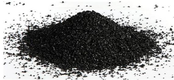
Gambar 1. *Copper Slag*
