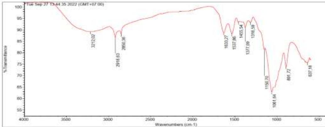
Figure 1. FTIR Spectrum of chitosan extracted from pupae shell of maggot waste without  $H_2O_2$  immersion with DD 75.3 %
