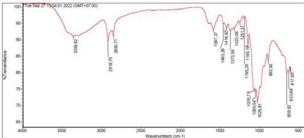
Figure 3. FTIR Spectrum of chitosan extracted from pupae shell of maggot waste with  $H_2O_2$  15% with DD 78 %
