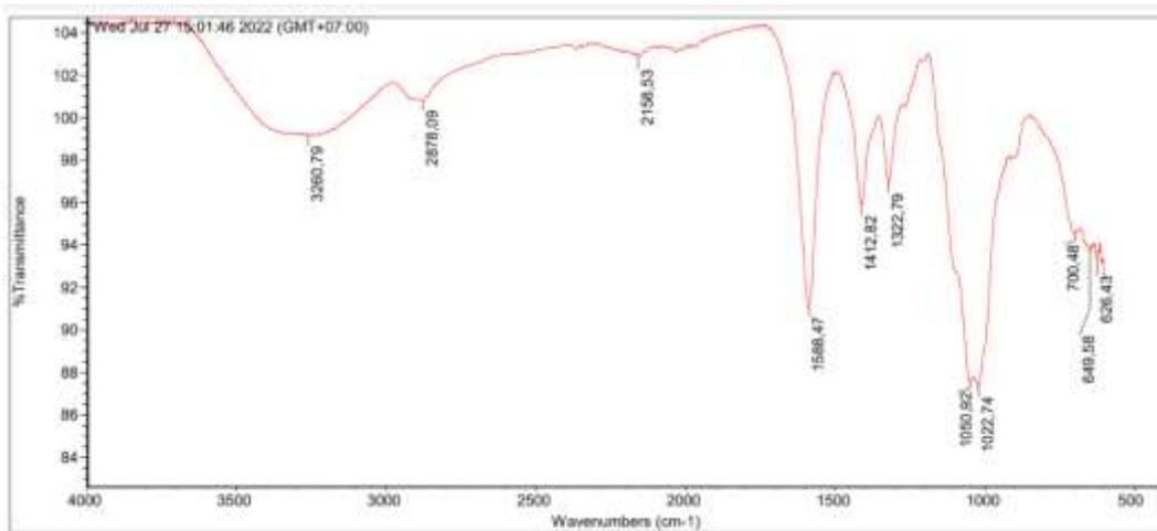
Figure 5. FTIR Spectrum of commercial chitosan at DD 84%
