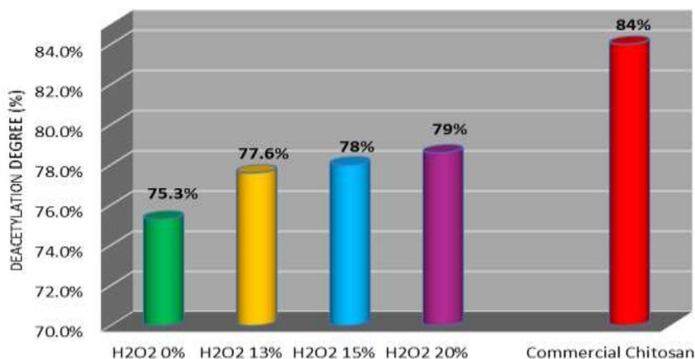
Figure 6. Deacetylation degree of chitosan extracted from pupae shell of maggot waste and commercial chitosan
