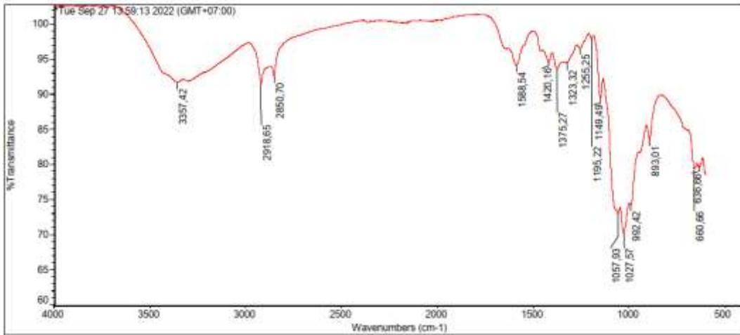
Figure 4. FTIR Spectrum of chitosan extracted from pupae shell of maggot waste with H<sub>2</sub>O<sub>2</sub> 20% with DD 78.6 %
