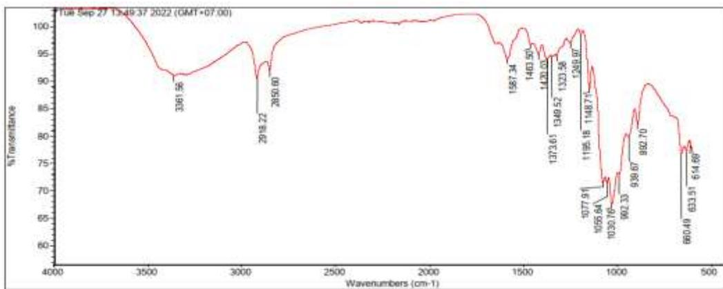
Figure 2. FTIR Spectrum of chitosan extracted from pupae shell of maggot waste of  $H_2O_2$  13% with DD 77.6 %
