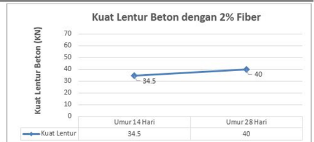
Gambar 7. Kuat Lentur Beton 2% Fiber Polypropylene Sumber: Hasil pengolahan data
