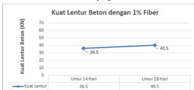
Gambar 6. Kuat Lentur Beton 1% Fiber Polypropylene Sumber: Hasil pengolahan data
