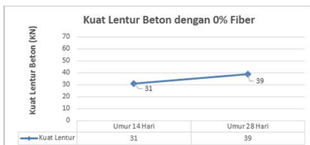
Gambar 5. Kuat Lentur Beton 0% Fiber Polypropylene Sumber: Hasil pengolahan data
