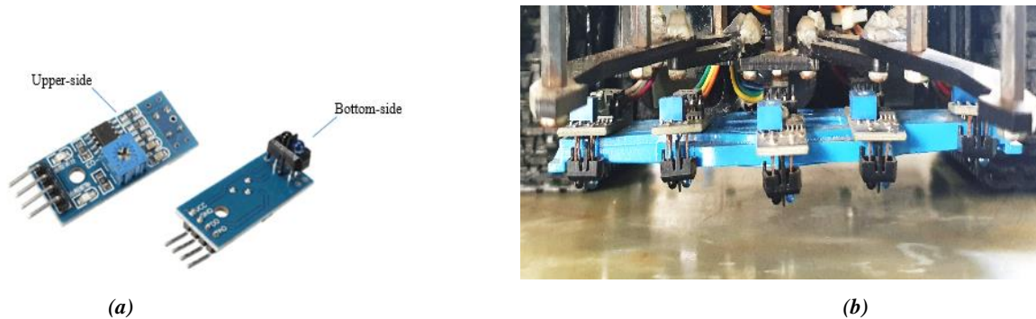
Fig.3. (a)The TCRT5000 Modules Infrared Sensor; (b)Placement of 5 Modules TCRT5000 Sensors at The Bottom of The Forklift Robot
