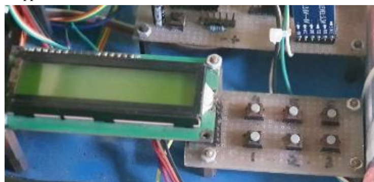
Fig.5. The layout of Keypad and Liquid Crystal Display (LCD) Alphanumeric
