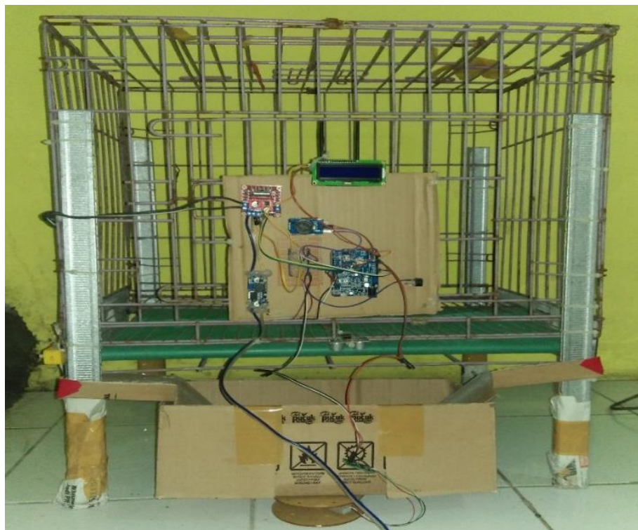
Fig. 4. Prototype Of A Rabbit Cage With An Automated System For The Disposal Of Feces And Urine
