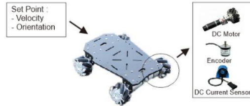
Figure 5. The mobile robot configuration
