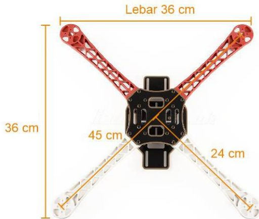
Figure 7. F450 quadcopter model design
