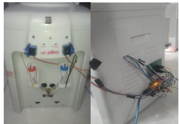
Figure 11. Automatic water dispenser based on gesture detection.
