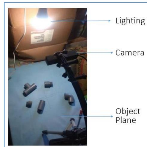
Figure 4. Environmental setup
