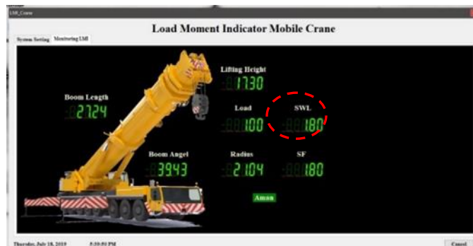
Figure 18. Mobile Crane Display in Computer
