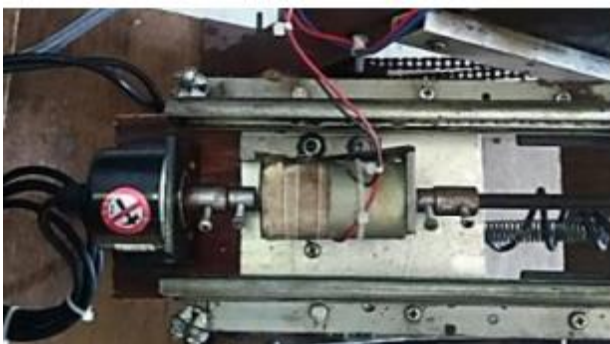
Figure 14. Rotary Encoder Installation
