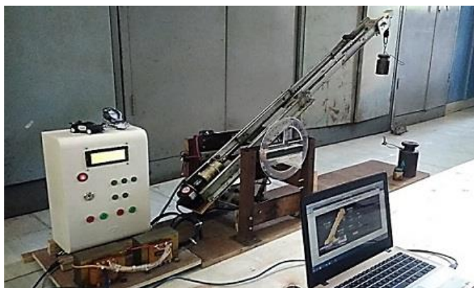
Figure 9. Desain of LMI Prototype On Mobile Crane
