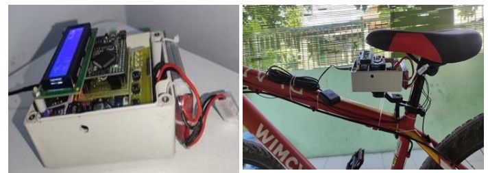
(a) Board Controller Placed Inside A Box (b) The Box Placed Electronic On The Bike
