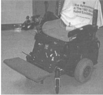
Gambar. 1 *Autonomous Robotic Wheelchair*[6]
