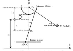
Figure 4. Hyperbole omnidirectional mirror model
