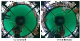
Fig 12. Goal detection result using radial search lines
