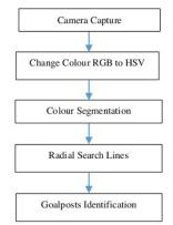
Figure 6. Goal Detection Process Diagram
